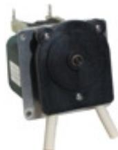
The 810 series peristaltic pumps are available in a range of 115v (MOQ applies) or 230v AC motor options with shaded pole gear motor and plastic cooling fan (not 30RPM). Capable of delivering flow rates as high as 987 ml/min, the pump heads are Clear Polycarbonate as standard with a black polypropylene option (shown in picture). The 810 pump is supplied with stainless steel fasteners. All AC models run clockwise.
