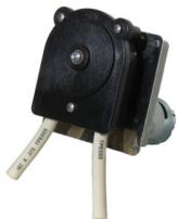
The 810 series peristaltic pumps are available in 12 or 24v DC motor options. They are capable of delivering flow rates as high as 987 ml/min, the pump heads are polypropylene with stainless steel fasteners, self priming from dry 5 metres, pressures up to 20 psi (1.5 bar), are non-siphoning and can be run dry continuously.
