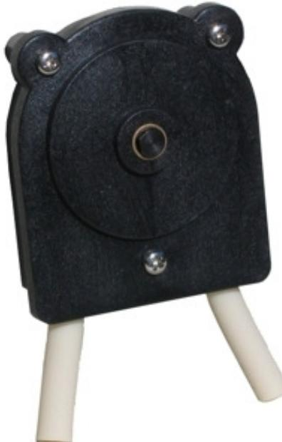
The 810 series of peristaltic pumps are capable of delivering flow rates as high as 987 ml/min, the pump heads are polypropylene with stainless steel fasteners, self priming up to 29 ft. (8.8m), run up to 20 psi (1.38 bar), are non-siphoning and can be run dry continuously.
