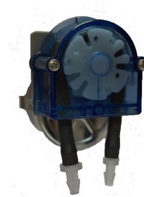
The 200 series, range of peristaltic pumps offer a low cost, compact & reliable means of dosing a wide range of liquids. They are available in various configurations of tubing type & size giving flow rates of between 0.1 & 1.32 ml/rev. The pump head is designed to be disposable but is assembled using a single screw enabling dis-assembly & re-assembly for tube changing if required.
