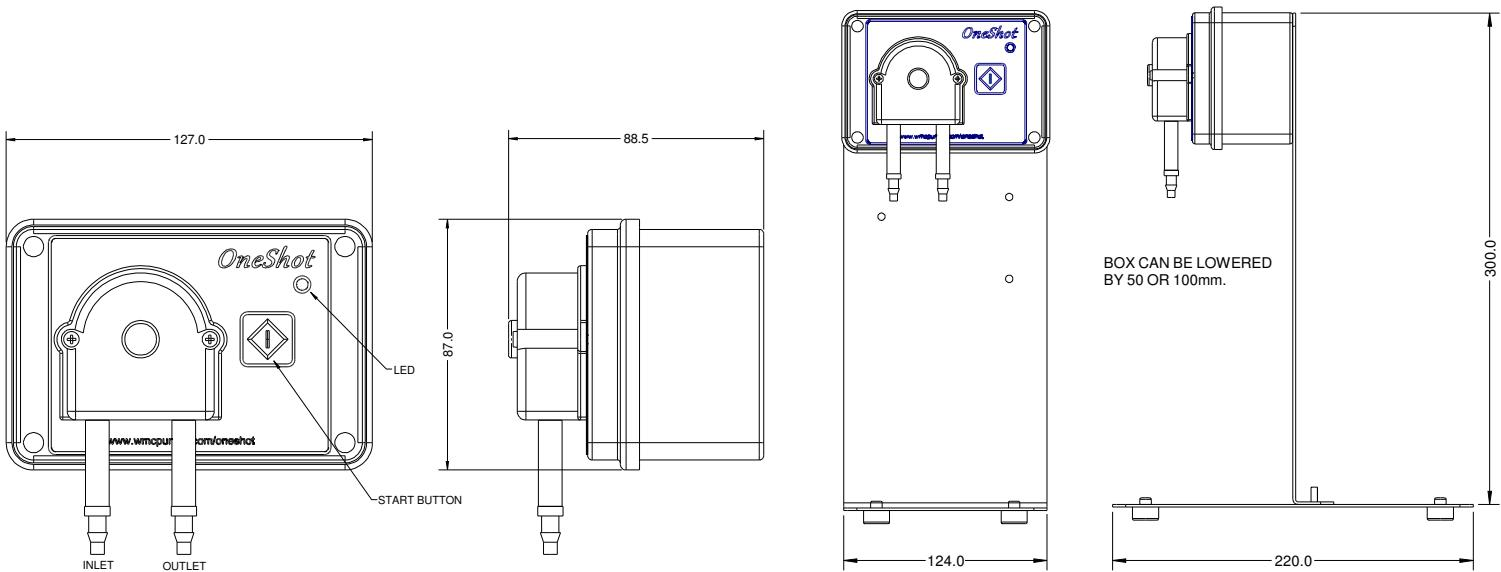
Important: The standard version of this pump is supplied sealed so the tube cannot be changed. The pump has been designed so that when the pump head has worn out it is changed as a whole. We are able to supply pumpheads unsealed for customers that wish to change the tubing periodically. Please contact our office for details.
