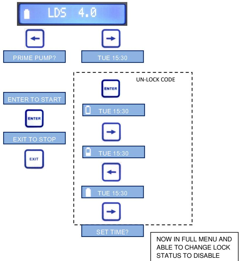
NOTE : IF BACK UP BATTERY IS NOT FITTED OR IS DISCHARGED WHEN THE MAIN BATTERY IS CHANGED OR RE-FITTED THE TIME WILL NEED TO BE RE-SET OR DOSES COULD OCCUR AT THE WRONG TIMES.
