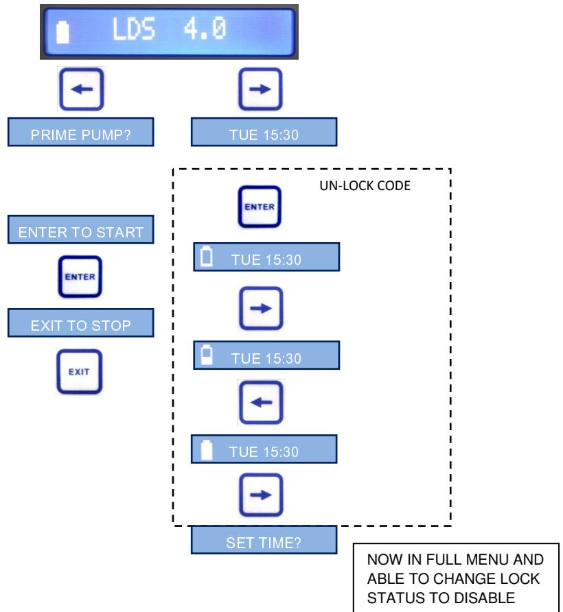
NOTE : IF BACK UP BATTERY IS NOT FITTED OR AFTER SIGNIFICANT OR MULTIPLE MAINS FAILURE(S) THE TIME WILL NEED TO BE RE-SET OR DOSES COULD OCCUR AT THE WRONG TIMES.
